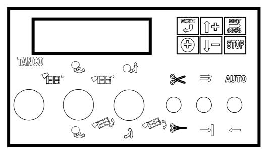
The TANCO wrapper machine controller is an advanced automatic system. It both control and monitors the moving machine parts and thereby provides for an optimal efficient and safe machine operation. The system gives detailed instructions and messages via the 40 character alphanumeric display, enabling the operator to monitor the operation of the wrap machine at any instant.
