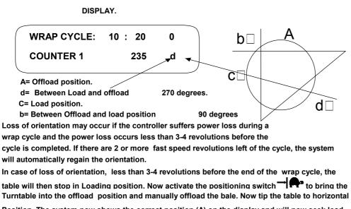
Position. The system now shows the correct position (A) on the display and will now seek load position ( C ) on the next auto start command.
