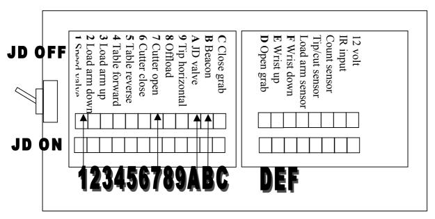
The cutter open function requires that terminals 1,7,A AND B, present 12-volt on their respective outputs when the function is active. Note that the A terminal is the JD function with an inverted output, meaning that the terminal when inactive presents 12 volt on the terminal and is ground when active.
