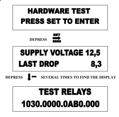
When testing a function e.g. Table rotate, a number of outputs are activated simultaneously as other devices usually are required activated at the same time such as the beacon and slow speed during the start of the wrapping cycle. In the above example the loading arm down function is active. The output no 1 is the Two speed valve ( high speed ), 3<sup>rd</sup>. output is the load arm down function, A ( terminal output No.10 ) is the beacon and B (No. 11 ) is the JD. Output terminal.
